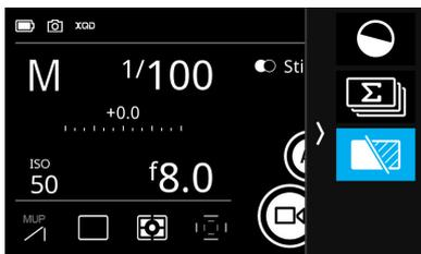
Once you have entered Dual Exposure+, the Aperture, ISO value and Shutter Speed can be set. Note how the secondary exposure is automatically set be three stops longer - the calculated exposure time is displayed under the Shutter Speed in grey.
