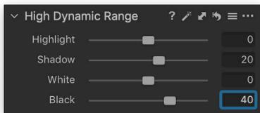
The two captures are kept separate and bundled into the same RAW file to achieve the best possible image quality once they are combined in Capture One. In the software, the wider dynamic range will be realized and become visible once you start to recover the shadows areas with the **Shadow** and **Black** sliders in the **High Dynamic Range** tool.
